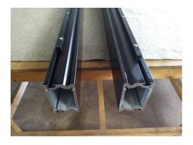
Flip your extrusion over. Slid (3) t nuts into each slot. Locate your drag chain mounts (2). Use m5x12 button caps screws to attach the drag chain mounts to the t nuts. The Drag chain mounts has a slot on one side that should be positioned to the "back" of each extrusion.
