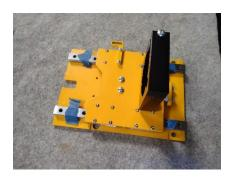
Prop the x plate on its bottom using the router mount. Place eccentric spacers in the top, large holes on the back of the x plate. Insert m8x40 machine screws into the large holes in the front of the x plate and through the eccentric spacers. Place an assembled v-wheels on the M8x40 machine screw and secure with a m8 nylock nut.
