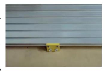
to the other end of the shorter 2040 extrusion. Attach the mid-span joiner plate to the bed using (2) m5x12 button cap screws.
