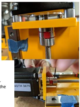
Locate the X/Y motor mount and lower the z plate to expose the two holes near the center top of the x plate. Place a m4 split lock washer on (2) m4x12 machine screws. Insert the screws through the front of the x plate and attach the X/Y motor mount to the back of the x plate.
