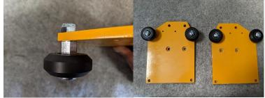
Place a v wheel on an m8x40 machine screw. Place a standard spacer on the m8x40 machine screw and place the screw through the bottom set of holes on the front of the right Gantry End Plate. Secure with a m8 nylock nut. Repeat the process with the left Gantry End Plate.
