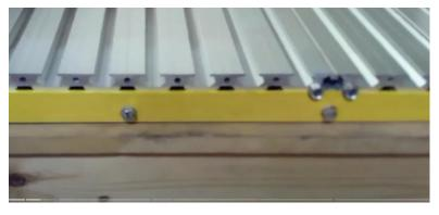
the "front" of the bed and the small section at the "back". Order does not matter on the Mega V 35x35. Make sure the top of the bed sections are showing; the side with the large, numerous slots is the top. The top holes of the Bed Joiners should match up with holes on the side of the bed sections. Connect the joiners with the bed sections using #10 x 1" self tapping screws. WD40 or other lubricants can be used to easy the cutting of the threads. Leave the screws loose.
