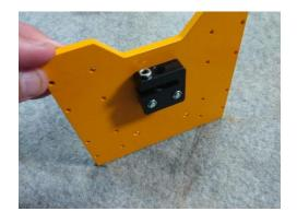
Locate the z rails with bearings. The bearings will slide off the rails expelling all ball bearings. Please proceed with caution. The rails will have plastic or rubber blocks to keep the bearings from sliding off. Leave them in place until told to remove them. If the blocks are not present, tape both ends of the rails to keep the bearings from sliding off. Place the z rails on a flat surface with the bearings face up.
