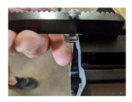
Retrieve the x/z assembly. The v-wheels will pinch the outside of the Mega V extrusion using the v shaped slots on the top and bottom. If the v-wheels are too tight to slide on the extrusion, use a 13mm wrench to turn the eccentrics until the assembly slides onto the extrusion.
