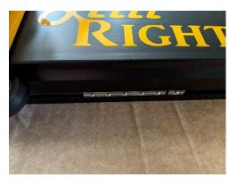
Retrieve the left end plate. On the left side of the extrusion, use (4) 5/16 x 3/4 button cap screws to attach the left end plate to the extrusion. Repeat the process on the right side with the right end plate. The end plates should extend more from the front of the extrusion than the back.
