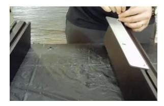
Slide the gantry onto the y extrusion. The v wheels should fit in the groove on the extrusion. If the fit is tight, use a 13mm wrench to rotate the eccentric spacers to loosen the fit. Make sure the rack on the extrusion is facing up. Do this for both extrusions.
