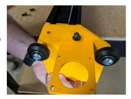
Tilt the gantry forward to gain access to the bottom. Using (3) m5x12 button cap and the installed large t nuts, attach the drag chain mount. The drag chain mounts need to be positioned on the right side of the gantry as seen from the front with the slotted ends pointed out towards the end plates. Leave loose. Please be careful not to bend the drag chain mounts. Set the gantry to the side.
