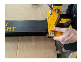
Slide (3) large drop in t nuts into the bottom slot of the Mega V extrusion. (6 t nuts shown in picture – only use 3)
