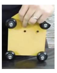
Locate a X/Z Motor Mount. The mount will be installed on the same side of the Gantry End Plates as the v-wheels. Place (2) M4x12 machine screws through the back of the Gantry End Plate (opposite the v-wheels) using the two small holes located between the v-wheels and install the motor mount. Repeat the process on the other Gantry End Plate. Place both to the side.
