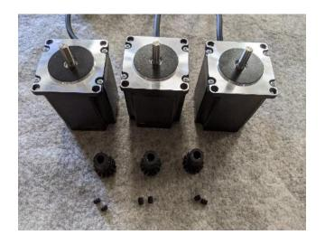
Locate the pinion gears (3) and the motors (3). The set screws are in the bag with the pinion gears. There are two screws for each pinion gear. Slide the pinion gear over the shaft of the motor and secure with the set screws. Have one set screw over the flat section of the motor shaft for a more secure hold. Repeat the process for the remaining motors.
