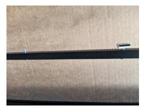
Slide the t nuts into the top of the Mega V extrusion with the gear rack teeth pointing towards the back of the extrusion. The Logo is on the front of the extrusion. Leave the rack loose.
