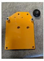
Repeat the Process with the Left Gantry End Plate. The recessed pockets on the plate should be face up.
