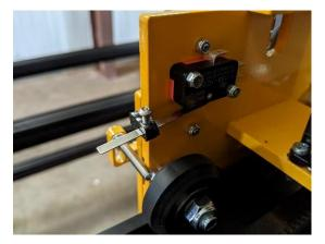
Slide the small black extender piece onto the paddle of the switch and secure it in place by threading an M3x8 machine screw into the plastic.
