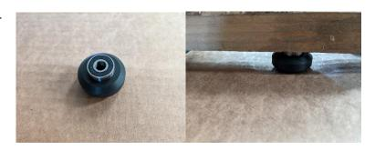
Flip the v-wheel over. Place a M8 washer flat on the 608 bearing inside the v-wheel. If you forget this step the bearing will not spin correctly. Correcting this will be difficult.
