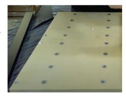
Locate the long 2040 extrusion (2). Slide the extrusion over the (4) t nuts on the edge of the bed sections. On the 19x19" Mega V, the extrusion is flush with the side edge of the bed sections. On the 35x35" Mega V, the extrusion should extend over the side edge of the bed sections. You will repeat the process with the short 2040 extrusions and the middle T nuts. Make sure the bed sections are pressed together firmly and even. Tighten the m5x18 machine screws.
