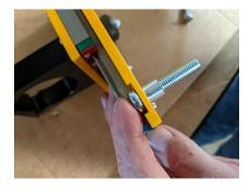
Thread the 178mm lead screw into the ABN. Locate the z motor mount. Using (2) m4x12 machine screws with m4 split lock washers, attach the z motor mount to the top of the x plate.
