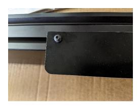
Locate the gear rack (2) and the 1064 Mega V extrusion (2) for the XL, or (2) 670 Mega V extrusion for the standard size. Insert m5x20 machine screws through the holes of the gear rack and lightly thread t nuts on the screws. Slide the t nuts into the slot on the Mega V extrusion with the teeth facing out of the extrusion.
