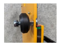
Place (2) m8x40 machine screws in the large holes in the front of the x plate at the bottom. Place standard spacers on the m8x40 screws, assembled v-wheels, and secure with a m8 nylock nut.
