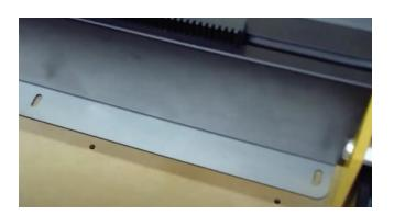
On the Y axis, make sure the slots on your drag chain mounts are positioned to the back of your machine as viewed from the front. Secure the drag chain with a m4x12 machine screw and nylock nut.
