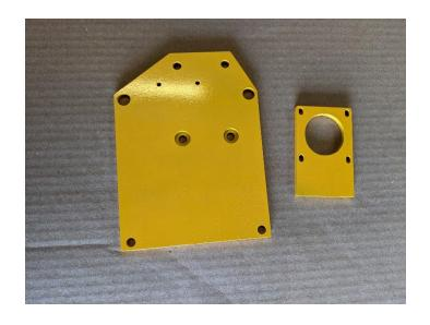
We have recently changed the XY motor mounts. The one on the right with the threaded screw holes is the older style and will have instructions after this section. The one on the left with the slotted holes is the new style with instructions in this section. There will be another division of instructions when mounting the XY motor mount on the X plate and mounting the XY motors.
