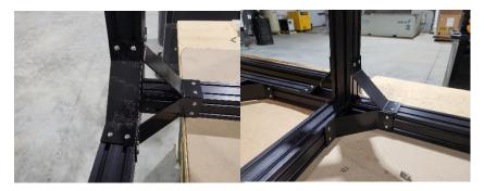
The 2650 Extrusion and the front/rear 1465 extrusion will need (2) corresponding t nuts for each set on the legs.
