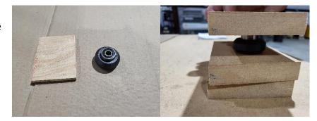
Flip the v-wheel over. Place a M8 washer on the 608 bearing inside the v-wheel. If you forget this step the bearing will not spin correctly. Fixing this will be difficult.
