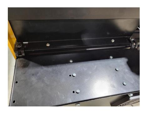
Place (4) Drop-in t nuts in the top outside slot of the right 2650 frame extrusion near the front of the machine. Using (2) M5x12 button caps with M6 washers, attach the box to the side of the machine using the first and last drop in t nuts. The Red estop button on the box should be facing the front of the machine.
