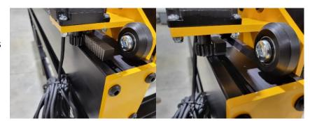
Starting with the left Y motor, gently push the motor to the rack and tighten the motor. Gently pull the rack to the motor and tighten the front screw on the rack. Continue moving the gantry down while gently pulling the rack to the motor and tightening the rack as you go. Repeat the process with the right Y motor, and then the X motor starting at the right as seen from the back of the back of the machine.
