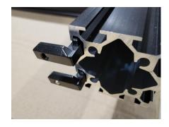
Slide the 1465 extrusion into the 2650 extrusion. Repeat the process with (5) of the remaining (6) 1465 extrusion. Keep the corner joiners pointing the same way, towards the opposite end of the 2650 extrusion. The spacing of the extrusion is about 371.66mm (14 5/8") between the extrusions. The last extrusion should be inserted into the other end of the 2650 extrusion with the corner joiners pointing towards the opposite end.
