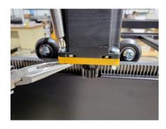
Set a 4750 motor on the X motor mount on the back of the gantry with the wire facing the rear of the machine. When looking at the motor from the back of the machine, the two motor holes on the left will receive M5x16 machine screws. The two motor holes on the right will receive M5x20 Machine Screws. Slip the Drag Chain Mount onto the M5x20 machine screws with the slot facing to the right. Secure with M5 Nylocks. Leave loose to adjust the rack.
