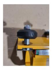
Locate the Z motor mount. Use the Z motor mount as a spacer for installing the coupler onto the 4750mm motor. Tighten the pinch screw on the 6.35mm side of the coupler to attach the coupler to the motor shaft.
