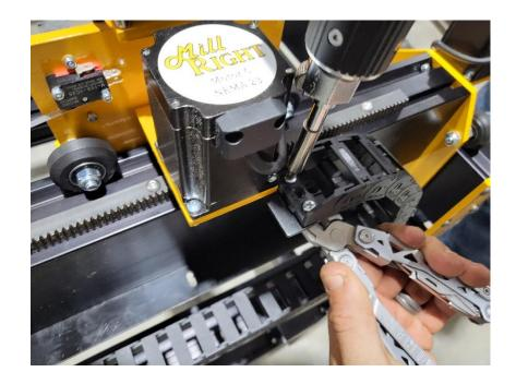
Locate the short drag chain. Disconnect the last link on one side, flip the link over, and reattach the link to the chain. Attach that end to the top of the drag chain bracket on the X motor mount with (2) M4x12 Machine Screws and (2) M4 nylock nuts. Stretch out the drag chain and open all the gates on the back of the drag chain. If the gates come off, just store them somewhere until needed.
