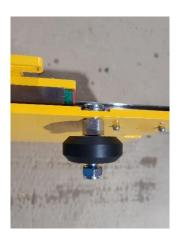
Place (2) M8x40 machine screws in the large holes in the front of the X plate at the bottom. Place standard spacers on the M8x40 machine screws, assembled v-wheels, and secure with a M8 nylock nut.
