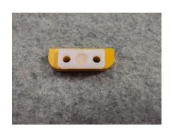
Secure the UHMW screw seat to the screw seat plate using (2) M5x16 machine screws and (2) M5 nylock nuts. Do not over tighten or you may deform the UHMW screw seat.
