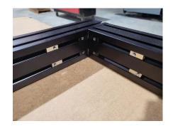
Using the M5x8 Button cap screws, attach the gussets to the 1465 Extrusion and the 2650 extrusion. There will be (2) gussets for each 1465 extrusion, one on either end, for a total of (14) gussets.
