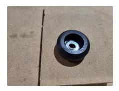
Place a second 608 bearing on top of the v-wheel. Press the bearing into the v-wheel using your impromptu tool. Pinch the inner races of both bearings with your fingers and test that the v-wheel spins freely. Repeat this process with the remaining v-wheel bodies. Set the v-wheels to the side.
