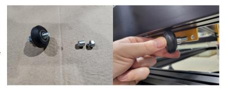
You may need to adjust the eccentric spacers on the top v wheels to allow the bottom v-wheels to be installed. Use a 13mm wrench to rotate the eccentric spacer to allow the plate to drop to the lowest point. The eccentric spacers have a flat spot on one corner to denote The highest position of the plate. Put the flat spot on the bottom for the lowest plate position. Continue installation with the remaining v-wheels.
