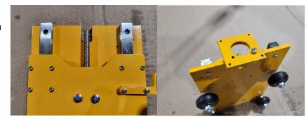
Locate the X/Y motor mount and lower the Z plate to expose the two holes near the center top of the X plate. Place a M4 split lock washer on (2) M4x12 machine screws. Insert the screws through the front of the X plate and attach the X/Y motor mount to the back of the X plate.
