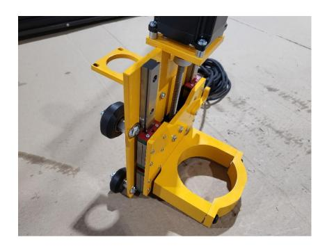
Locate the 4750mm Motor with coupler. Place 6.35mm spacers (4) on the mounting holes of the Z motor mount. Place the 4750mm motor with the motor wire positioned to the back of the X/Z assembly, opposite of the router mount, onto the spacers. Secure with (4) M4x16 machine screws.
