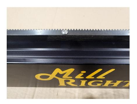
Get one section of long gear rack. Place M5x20 Button cap screw through the holes (12) of the gear rack keeping the screws uniform. Spin a large t nut a few turns on each screw. Leave the t nuts loose. Repeat process for the remaining long gear rack and the short gear rack.
