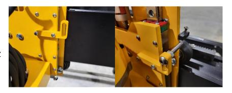
Locate the long roller switch and a L bracket. Place the red part of the switch on the L bracket with the roller facing the flat side of the L bracket. Place (2) M3x20 machine screws through the black side of the switch and secure with (2) M3 nylock nuts.
