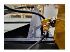
Curl The drag chain towards the front of the machine. Connect the end of the drag chain to the slot in the front most drag chain mount using a M4x12 machine screw and a M4 nylock nut.
