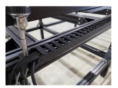
Move the gantry all the way forward. Zip tie the drag chain to the slot on the second drag chain mount attached to the 2650 frame extrusion before the chain curls up.
