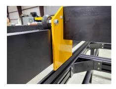
Once the wheels are installed. Move the gantry back and forth. The travel should be smooth. If one side lags, the wheels are too tight. Each v-wheel should rotate when the gantry is moved, but you should be able to rotate each wheel individually with your fingers.
