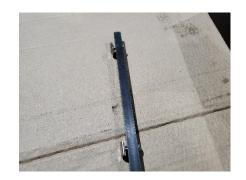
Slide the t nuts into the top of the Mega V extrusion with the gear rack teeth pointing out from the extrusion, away from the v groove. Leave the rack loose. The (2) 2650 Mega V extrusions will get the long rack. The 1465 Mega V Extrusion w/logo will get the short rack.
