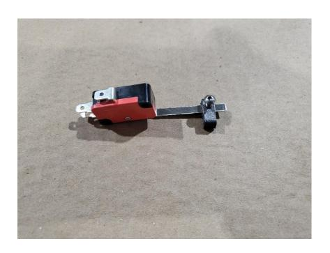
Locate the long paddle switch. Locate printed extender piece. Slide the extender onto the paddle with the screw hole facing the switch and the printed extender out towards the red side of the switch (shown above). Insert a M3x8 button cap screw to secure the printed extender to the paddle.
