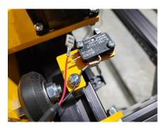
The homing wires are marked near the end close to the spade connectors. The black wire will connect to the terminal exiting the side of the switch and curving down, pictured above. The red wire will connect to the terminal closest to the black terminal. Connect the Z and X switches. Leave the Y switch alone for now.
