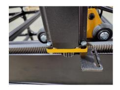
Place the 2550 motor on the right Y motor mount with the wire pointing to the rear of the machine. When looking at the motor from the right of the machine, the two motor holes on the left will receive M5x16 machine screws. The two motor holes on the right will receive M5x20 machine screws. Slip the Drag Chain Mount onto the M5x20 machine screws with the slot facing to the right. Secure with M5 Nylocks. Leave loose to adjust the rack.
