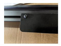
Locate the (2) Y mid-span supports. In the middle of the 2650 Mega V extrusion (1325mm), opposite the rack, place (2) drop-in t nuts in each extrusion. Place M5 split lock washers on (4) M5x25 button cap screws. Attach the Y mid-span supports to the 2650 extrusion using the M5x25 button caps with split lock washers and the drop-in t nuts. Orientation of the Y mid-span support does not matter.
