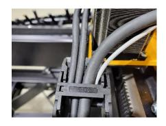
Do not run the left Y Motor Wire through the X Drag Chain. Close the gates.
