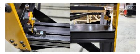
Locate the short roller switch and a L bracket. Place the red part of the switch on the L bracket with the roller facing the flat side of the L bracket. Place (2) M3x20 machine screws through the black side of the switch and secure with (2) M3 nylock nuts.
