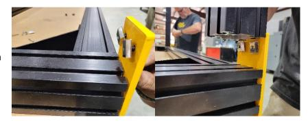
Place (2) drop-in t nuts in the grooves of the legs, one in each slot, for each face of the leg that is perpendicular to the 2650 extrusion and the front/rear 1450 extrusion. There will be (4) drop-in t nuts for each leg total. Use M5x8 button caps to install gussets on the legs using the drop-in t nuts. There will be 2 gussets for each leg.
