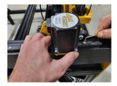
Once the rack is tightened, move the gantry back and forth checking for smoothness. If you feel any tight spots in the travel, loosen the screws near the tight spot and apply a bit of pressure to the rack to move it away from the pinion gear slightly. Retighten the rack and continue checking the travel.
