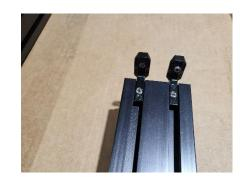
Slide the 1465 extrusion into the front set, middle set, and rear set of legs. Sit them on the gussets. Slide the
