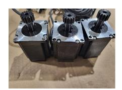
The 4750 motors will go on the left Y axis and the X axis on the back of the gantry. The 2550 motor will go on the right Y axis.
