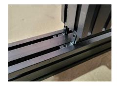
Place (2) M5x16 button cap screws through the outside of the y end plate and lightly thread on a large t nut to each screw. Slide a 760 leg extrusion onto the t nuts. Tighten the M5x12 button caps while making sure the leg is flush with the outside of the 2650 extrusion. Repeat for the other y end plates and legs.
