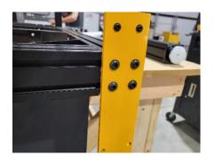
Slide (2) 760 leg extrusions onto the inside corner joiners, one leg extrusion for each 2650. There are two tapped holes diagonally from each other on one end of the 760 extrusions. Make sure the tapped holes on the 760 extrusions are pointing up. Leave the legs loose. The legs will need to be adjusted when installing the subframe. Leave the legs near the center of the 2650 extrusion.
