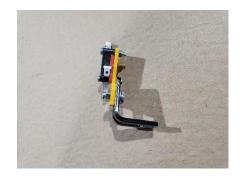
In the top of the rear 1465 Extrusion, in the first slot, place a drop-int nut. Secure the 90\* slot to the 1465 extrusion using a M5x12 machine screw with a M5 split lock washer. The edge of the right gantry end plate (on the left as viewed from the rear of the machine) should engage the switch near the end of travel. This is the Y switch.
