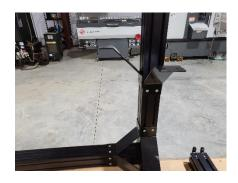
Preload the set screws in the inside corner joiners. (2) set screws for each corner joiner. Side the corner joiners, (2) on each side - (4) in total, in the 1456 extrusion oriented where they terminate against the end of the 1465 extrusion. Repeat this process with the 1235 extrusion.
