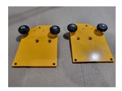
Locate a X/Z motor mount. The mount will be installed on the same side of the gantry end plates as the v-wheels. Place (2) M4x12 machine screws with a M4 split lock washer each through the back of the gantry end plate (opposite the v-wheels) using the two small holes located between the v-wheels and install the motor mount. Repeat the process on the other gantry end plate. Place both to the side
