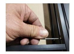
The gussets will connect the 1465 extrusion to the 2650 extrusion on the side opposite of the inside corner joiners. Place (2) drop-in t nuts, one in each slot, on each end of the 1465 extrusions for a total of 4 drop-ins for each extrusion. The front and back extrusions will have the gussets on the same side as the inside corner joiners. Place (2) corresponding drop-in t nuts in the 2650 extrusion for each set in the 1465 extrusion.
