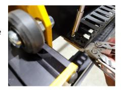
Locate the long drag chain. Attach the drag chain to the underside of the drag chain bracket on the right Y motor mount using (2) M4x12 machine screws and (2) M4 nylock nuts. Open the gates on the back of the drag chain and stretch out the chain.
