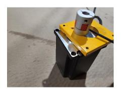
Thread the 178mm lead screw into the ABN. Using (2) M4x12 machine screws with M4 split lock washers, attach the Z motor mount to the top of the X plate.
