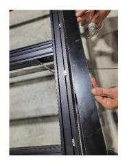
Loosen the (4) 5/16x3/4 button cap screws on each of the Y end plates. Locate the right Mega V Y rail (with the drag chain mount installed). Place between the right Y end plate, with the rack on the outside of the rail and the rack teeth pointing out, and secure with (4) 5/16x3/4 button cap screws (pictured at top). Repeat the process with the other end of the Y end plate. While tightening the 5/16x3/4 button cap screws, check for
