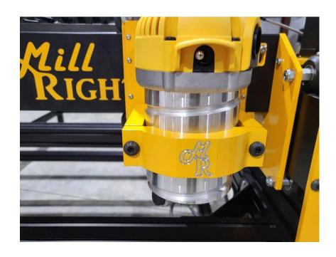
Take the DW618 router from the box and remove all plastic pieces from the barrel. Loosen the 5/16x1 button cap screws on the front of the router mount. Slide the 618 router into the router mount about 1/3 of the way up the barrel of the router. Make sure the on/off switch of the router is accessible from the front of the machine. Tighten the 5/16x1 button cap screws a little at a time until fully secure. Do not tighten one side down completely before tightening the other side.
