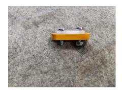
The front of the X plate is the face with the recessed pockets. The top of the X plate is the section with the "U" cutout, as shown above. Place the screw seat plate on the X plate near the bottom center set of holes. Make sure the UHMW screw seat is pointing towards the top of the X plate. Place a M4 split lock washer on (2) M4x12 machine screw and insert the screws
