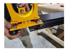
Retrieve the left end plate. On the left side of the extrusion, use (4)  $5/16 ext{ x}$  3/4 button cap screws to attach the left end plate to the extrusion. Repeat the process on the right side with the right end plate. The end plates should extend more from the front of the extrusion than the back. Set the 1460 Gantry to the side being carful not to bend the drag chain mounts.
