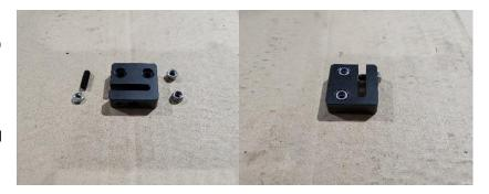
Cap the grub screw with the M5 jam nut. Place the ABN on the z plate and secure using the (2) M5x20 machine screws. Make sure the nylocks can be seen.
