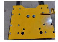
Locate the router mount. Carefully turn the Z plate on its side making sure the bearings stay on the rails. Place (2) 5/16x3/4 button cap screws through the back of the plate using the 2 large holes at the bottom of the Z plate. Attach the router mount to the Z plate and tighten the router mount screws. Use (2) 5/16x1button caps to attach the router cap
