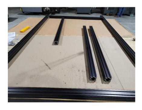
Preload the set screws in the inside corner joiners. (2) Set screws for each corner joiner. Screw them in from the inside of the v of the joiner. Make sure the set screw is not sticking out the back (outside v) of the corner joiner or they will not slide down the extrusion slots.
