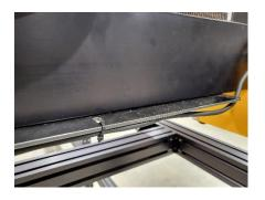
Curl the X drag chain around to the left (as viewed from the rear of the machine) and attach the end of the drag chain to the slot in the left most drag chain mount with a M4x12 machine screw and a M4 Nylock nut. Move the X/Z assembly all the way to the left. Zip Tie the drag chain to the slot in the second drag chain mount before the drag chain curls up.
