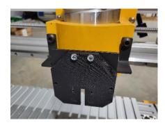
The laser will connect magnetically to the laser mount. The laser has 2 post on the back that will correspond with 2 holes in the lower middle of the laser mount.
