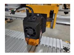
The laser diode is already enclosed with the fan already installed. The laser mount has magnets that allow the laser to snap to it. There are pins on the back of the laser that fit into corresponding holes on the laser mount.
