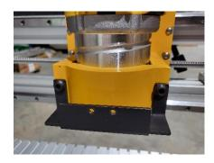
Using (2) M4x14 machine screws and (2) M4 nylock nuts, attach the quick connect laser mount to the outside of the laser bracket using the 2 small holes on the front. Make sure the laser mount is installed with the magnets to the back and the plain black surface facing out.
