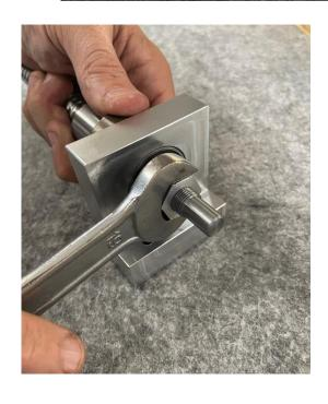
WARNING: Do NOT spin the ballnut all the way off the ballscrew. If you do, the ball bearings will fall out and the ball screw will have to be replaced.
