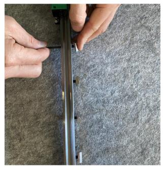
Place M5x16 button cap screws into the linear rail holes for the Y. Spin a "slide in" T nut onto each screw. Do not tighten the T nuts all the way against the rail as you will need to leave space to slide the nuts into the extrusion.
