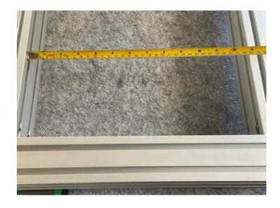
Use a square to make sure the crossmembers are perpendicular to the Y extrusions. Flip the assembly back over.
