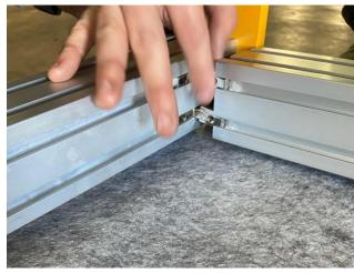
Continue to slide the 760mm crossmember extrusions onto the inside corner joiners. There are 3 crossmembers: front, middle, and rear. It is easiest to position all three in place on one of the Y extrusions, snug them into place on that side with the set screws on the joiners, then slide the other Y extrusion on.
