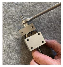
Slide the Z Floating Side Ballscrew Support onto the opposite end of the ball screw.
