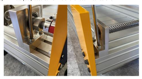
Install the Y ballnut housings onto the ballnuts using M5x16 button cap screws. The larger holes will face to the OUTBOUND side of the machine on both sides. Study the picture closely. It should look like this on both sides.
