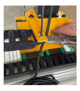
Tighten the coupler tensioning screws, making sure both the top and bottom screws are tight. Failure to tension these adequately will cause slippage during operation.
