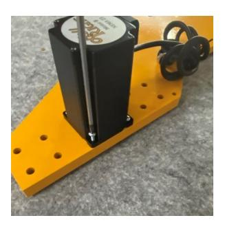
Install the remaining 6.35x10 coupler onto the shaft of the **B motor with the longer wire (2670mm)**, with the coupler about ¼" (6mm) from the face of the motor. Tighten the tensioning screw fully on the motor shaft.
