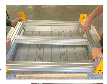
Use a straight edge to align the T Plate edges to the front crossmember.
