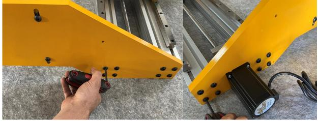
Place 4 drop in T nuts into the bottom slots of the bottom 888mm extrusion and install the side gussets with M5x12 Button Cap Screws. Then secure the Side Gussets to the Gantry End Plates with M4x20 Machine Screws.
