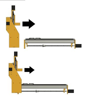
The gantry must now be set onto the lower frame. You can NOT set the gantry down onto the Y Bearings from the top. You must place the gantry onto the Y bearings from the back end. Use a helper with this step. Slide the Y bearings near the back of the machine so that you will not have to move the gantry as far when mating it to the lower frame.
