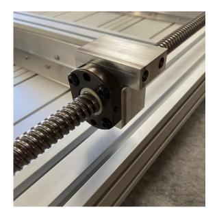
Flip the lower frame assembly back over, so it is in its "right side up" position. Remember not to let the bearings fly off the ends. Make sure your Y Ballnut Housings are in the configuration shown.
