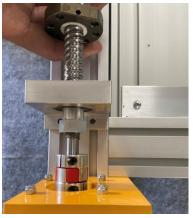
Tighten the Fixed and Floating Ball Screw Supports to the Y rail using M5x25 machine screws. These secure into the Large Drop in T Nuts you placed earlier. Do this for both Y ball screws.
