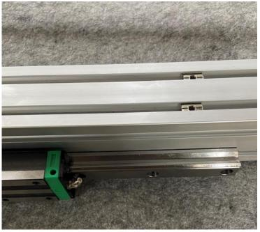
Note the position of the linear rail on this extrusion. Place the remaining 16mm ball screw assembly onto the rail.
