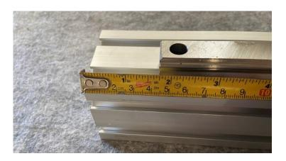
Just as you did with the other linear rails on the Y axis, place M5x16 button cap screws into the holes of the linear rails and spin Large Slide-in T Nuts onto the threads a couple of turns. Slide one linear rail onto each onto the 888mm extrusions. Tighten a couple of screws down to hold them in place about 1.75" (45mm) from the edge.
