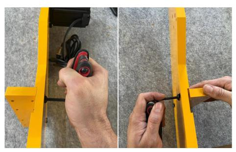
Install the Gantry End Plates onto the 888mm extrusions using 5/16"x1" button cap screws. Study the picture to the right closely so that you get the proper orientation of the top and bottom rails. Do NOT fully tighten either Gantry End Plate until both are installed and aligned.
