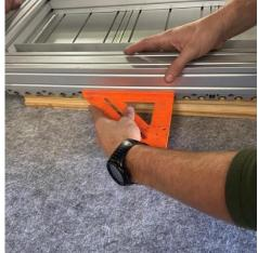
Place Large Drop in T nuts into the frame crossmembers in locations that correspond to holes in the corner joining angle (5 per angle).
