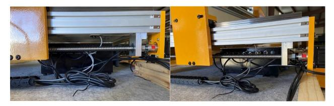
Plug the USB cable into the control box. Use a zip tie anchor and a zip tie to secure the wires coming from the Y drag chain, the left Y motor, the USB cable, and the box power cord on the left Y motor mount. Do this in such a way that the cables will not be rubbed by the coupler as it turns.
