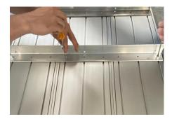
Install the final piece of table joining angle. Note the differing orientation of the flange.
