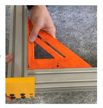
It can help to push the Y extrusions together to get the crossmembers more flush with the Y rails. You may need to loosen and retighten the set screws on the inside corner joiners to achieve squareness.
