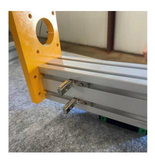
Slide one of the 760mm extrusions onto the inside corner joiner. Then slide the other end on.
