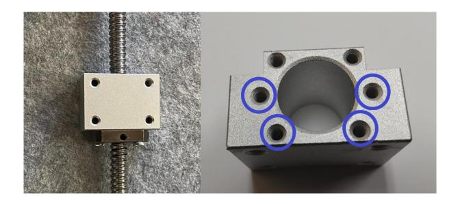
Slide the Z Fixed Ball Screw Support onto the threaded side of the Z Ball Screw. Seat it fully down, whacking with a mallet if necessary. Then spin the ballnut to the Fixed Side Ball Screw Support. Hold the assembly with your hand and tigthen the Z Preload Nut down with a 19mm or 3/4" wrench.
