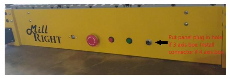
Note that it may be prudent to wait to install the side skirts and rear skirt until *after* you start the machine and begin moving it around. These panels protect you from pinch points at the table level of the machine, but any adjustments that need to be made to the system will require these panels to be removed. **They should remain installed during normal operation.**
