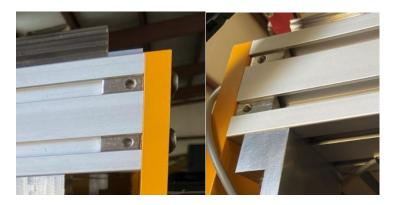
Slide the side skirts between the Gantry End Plates and the Y extrusions to get them into position. Secure them with M5x8 button cap screw.
