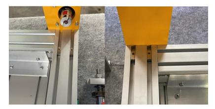
Place the ball screw assembly onto the Y rails. Push the shaft of the ball screw into the coupler.
