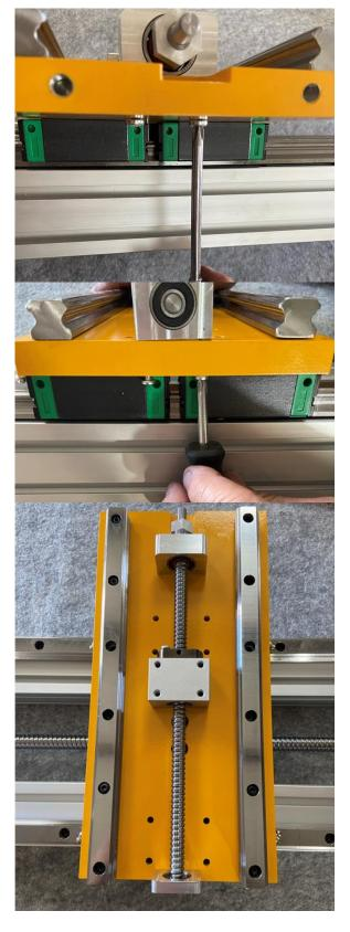
You'll now tighten the X rails down fully. Turn X the ball screw by hand to one end. Begin tightening all the hardware for the rails. Turn the screw some more and tighten the next set of screws until all the screws on the X Bearing Rails are tightened fully.
