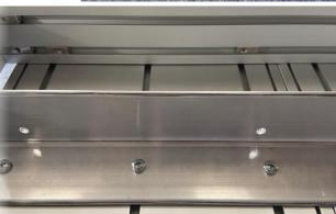
Slide the angle to the crossmember and fully tighten it with M5x12 machine screws. Do this for all positions, then fully tighten the M5x8 machine screws that hold the table joining angle to the T Plate.
