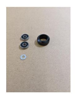
Press on bearing into a v wheel. Turn the wheel over, place a M5 washer into the wheel on the bearing, and press another bearing into the wheel. Do not forget the M5 washer. Repeat the process with the other 3 wheels.
