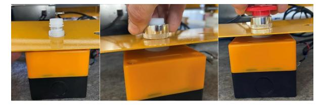
Install the red (pause) and green (resume) button into the holes in the panel. Put the red and blue wires on the terminals of the red switch. Put the green and black wires onto the terminal of the green switch. These wires can go on either terminal of their respective switch, so long as red and blue go to the red switch and green and black go to the green switch.
