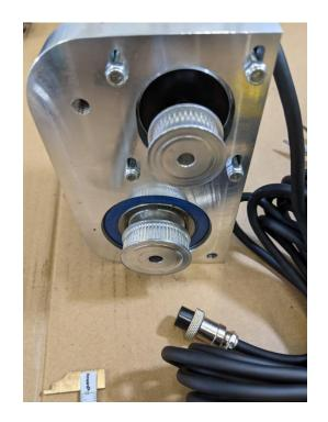
Place the belt on the gears smooth side out. Flip the chuck assembly motor side down to tighten the belt between the gears. Tighten the motor screws.
