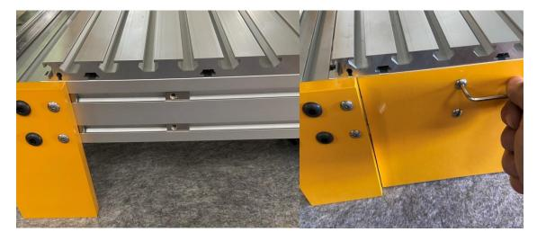
Each side skirt also installs with (4) drop in T nuts and (4) M5x8 button cap screws. Take careful note of how the thread holes in the drop in T nuts MUST face the outer ends of the machine. In other words, the T nuts need to be installed so that the hole is closest to the yellow plates at each end.
