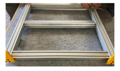
Once all three crossmembers are roughly in place, install the Y End Plate (looks about the same as the Y motor mount, but without the opening for the motor) using 5/16x3/4" button cap screws, secured into the pre-tapped holes on the Y extrusions.
