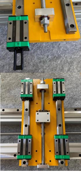
Place the Z Plate on top of the bearings. Line the bearings up as appropriate, and secure the plate to the bearings using M5x20 button cap screws. Note that the router mount will block one of the holes in each of the bottom bearings. This is expected.
