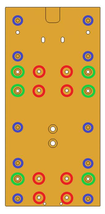
Place the Z Bearing Rails onto the X Plate. Some of the rails will have the bearings pre-installed. Others will not. Refer to page 2 for installation information if needed. Secure the Z Bearing Rails into place using M5x16 Button Cap Screws in the locations indicated by the **blue** circles above. Note that one of the holes in each rail will not receive a screw.
