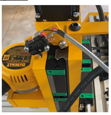
See the picture on page 29. Mount a short roller switch to a homing L bracket in the orientation shown using (2) M3x16 machine screws and (2) M3 nylock nuts. Install it onto the hole in the Z motor mount as shown in that picture with an M5x8 machine screw. Take note of the downward angle of the bracket. If it is not angled sufficiently downward, the homing switch will not be engaged by the Z axis plate during a homing cycle.
