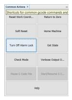
It the alarm comes from hitting a Homing switch, you will have to turn off the alarm lock and jog off the switch. May need to be done twice depending on your step size.
