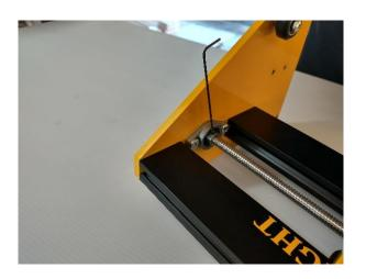
Use a Philips screwdriver to tighten the machine screws on the pillow block bearing. Use the 1.5mm Hex Key to tighten the set screw on the pillow block bearing. The coupler should NOT separate if you push the X/Z assembly to the right. If it separates, the set screws on the pillow block bearing are not set properly.
