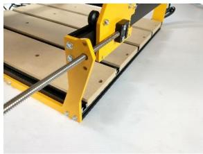
Continue to thread the lead screw back until the lead screw meets the coupler. Guide the screw into the coupler, tighten the set screw on the coupler, and fully secure the motor mounting screws. Repeat this for both sides.
