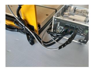
Note the approximate position for the control box. Also note where the USB cable and power cable plug into the control box. Power is brought to the machine simply by plugging and unplugging the power adapter barrel at this location.
