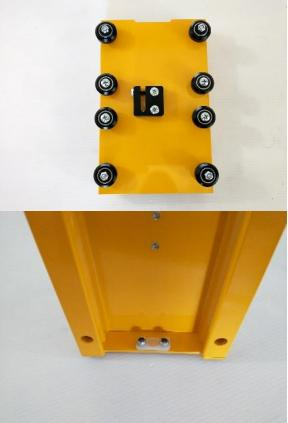
Attach the UHMW Screw Seat to the Z Bottom Plate using (2) M5x12 button cap screws and (2) M5 nylock nuts.
