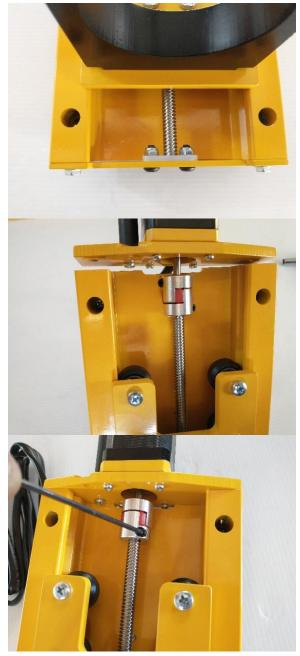
Using the 2.5mm Hex Key, tighten the coupler to the motor shaft and the lead screw. The lead screw MUST be firmly against the UHMW piece at the bottom of the assembly or the coupler will separate, causing the Z axis to lose height during operation. Make sure the coupler does not separate when the Z axis plate is pulled downward.
