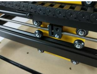
Place (2) 16mm (5/8") spacers onto the M5x50 bolt. Use the 8mm or 5/16" wrench or socket to screw the bolt into the hole that held the M5X16 machine screw in the anti-backlash nut.
