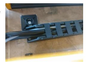
Grab some zip ties from the wire management bag. Thread the zip tie through the holes on the end of the drag chain and through the zip tie anchor. Place the electronics box near the end of the drag chain.
