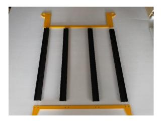
Lubricate 2 #10x1 self-tapping screws. Place the screws through the holes in the bottom of the frame into the holes in the end of the right most extrusion. Use the 8mm socket to drive in the screws. **Leave loose.** Continue installing the #10x1 screws in the other 3 extrusions.
