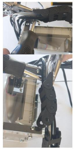
Note that the control box has been placed on its side to install these screws. After installing, set the control box back on its rubber feet and snap the drag chain back together.
