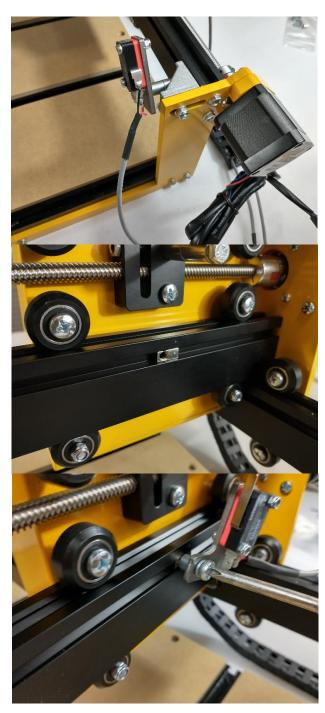
The Switch should be placed where it is triggered near the end of the X travel without being in the way of the Y switch. You can use spiral wrap (described in a later step) to secure the X axis switch wire to the cables coming from the X drag chain. This will secure it up and out of the way, preventing it from fouling the Y switch.
