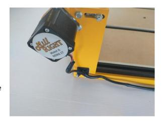
Run its wire to the back left and bundle the excess (there will be a fair amount of excess) to the back left of the frame along with excess from the back left Y motor. Secure it with zip ties and a zip tie anchor.
