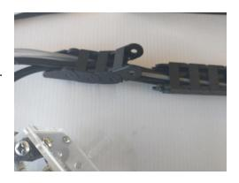
The control box has a slotted bracket already mounted to its underside. Mount the end of the cable chain to this using (2) M3x8 machine screws and (2) M3 nylock nuts. The head of the screw should closest to the wires and the nut on the other side.
