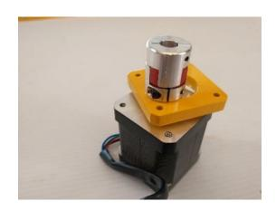
With the Motor Spacer Plate still on the motor, insert the coupler into the large hole on the Motor Side Y Gantry Plate. The motor wire should be pointing left if you are looking at the back of the motor. From the v-wheel side of the place (4) M3x16 machine screw through the Motor Side Y Gantry Plate, through the Motor Spacer Plate, into the motor. Snug down. Coupler should have free rotational motion.
