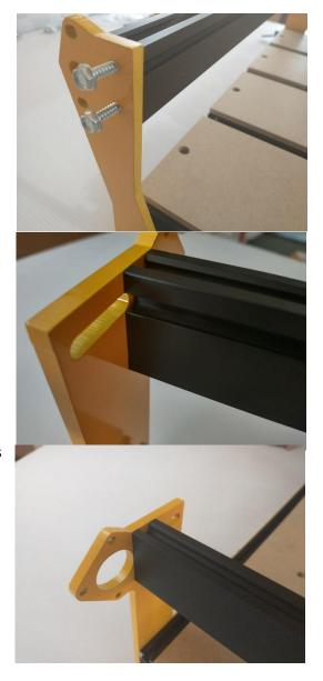
Lubricate (2) self-tapping screws. Place the screws through the two holes on the frame and into the holes in the end of the extrusion. Finger tighten the screws to hold the extrusion in place. Do the same to the other end of the extrusion. Follow the same process with the second extrusion on the other side of the bed. Be sure that the slots on the side of the extrusion faces inboard and are up.
