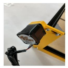
Thread a 600mm lead screw through the antibacklash nut on the right side of the Gantry using the large hole in the front frame. Keep threading until you insert the lead screw into the coupler. Repeat the process on the left side of the Gantry. Mini – You will have to install the pillow block bearing before threading in the 373mm lead screw. The bearings will need to be placed on the inside of the front frame, opposite of what is pictured on page 23 below.
