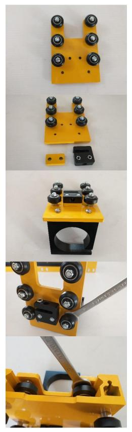
From the top of the X Plate Extrusion, thread the 178mm lead screw through the anti-backlash nut connected to the Z Plate. Continue until the lead screw is sitting in the pocket on the UHMW Screw seat.
