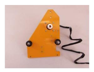
On the motor side of the Motor Side Y Gantry Plate, place an anti-backlash nut. Using (2) M5x16 machine screws, secure the anti-backlash nut to the plate.
