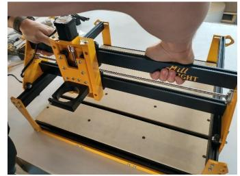
Place a V-wheel on an M5x25 machine screw, followed by a standard spacer from the V-wheel kit. Put the v-wheel into the V groove of the extrusion before tightening the screw. Screw the v-wheel into the bottom of the Gantry Y Plate. It the fit is tight, use the 10mm wrench to adjust the eccentric spacers. You may have to loosen the screws on the top wheels to get the bottom wheel screws to line up with the threaded hole.
