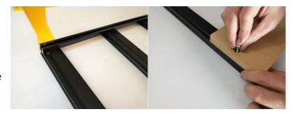
Alternate between the remaining T track and bed sections pushing each back.
