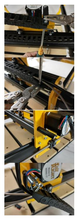
Locate the drag chain mount in the wire management kit. Remove the backing to expose the adhesive bottom. Attach the drag chain mount to the table near the back of the Carve King 2. The free end of the drag chain will attach to this point.
