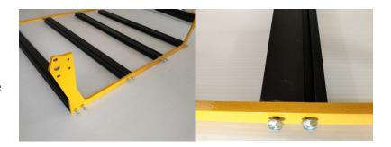
Spin the frame around to work from the other side. Put one drop-in T nut in each slot with the hole leading. Line up one T track with the T nuts. Using the 3mm Hex Key, drive in (4) M5x8 button cap screws. Leave loose. Push the t track to the frame. The hole of the T nut must be closer to the frame when slid all the way down or else the T track will not seat all the way to the frame.
