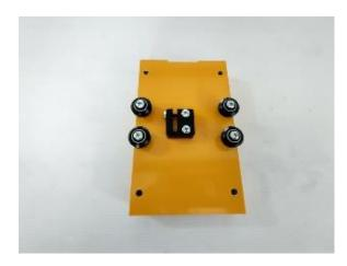
Screw an M5 grub screw into the top of an antibacklash nut using the 3mm Hex key. Cap the grub screw with a M5 Jam Nut. Using M5x16 machine screws, attach the anti-backlash nut to the X Plate Extrusion.
