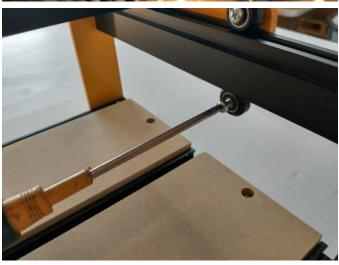
Insert a drop-in T nut into the Y Extrusion near the Rear Frame as pictured. Grab a corner bracket. If it has a tabbed side and a non-tabbed side, the tabbed side will fit into the slot on the Rear Frame as pictured. It is okay if neither side has tabs.
