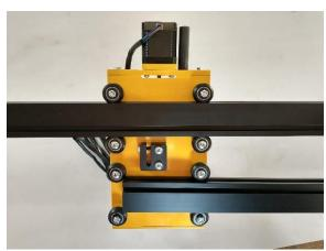
Lubricate (4) #10x1 self-tapping screws and place them through the Idler Side Y Gantry Plate into the holes on the end of the 613mm extrusion. Use the 8mm socket to tighten the screws.
