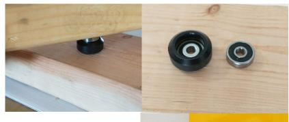
M5 nylock nut. Leave Snug, not tight. Repeat the process with another v-wheel. Take careful note of which side of the place the spacers and wheels are installed on.
